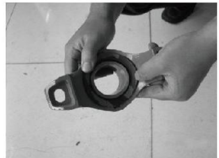
3. Put gasket seal in the Mechanical Tee.
